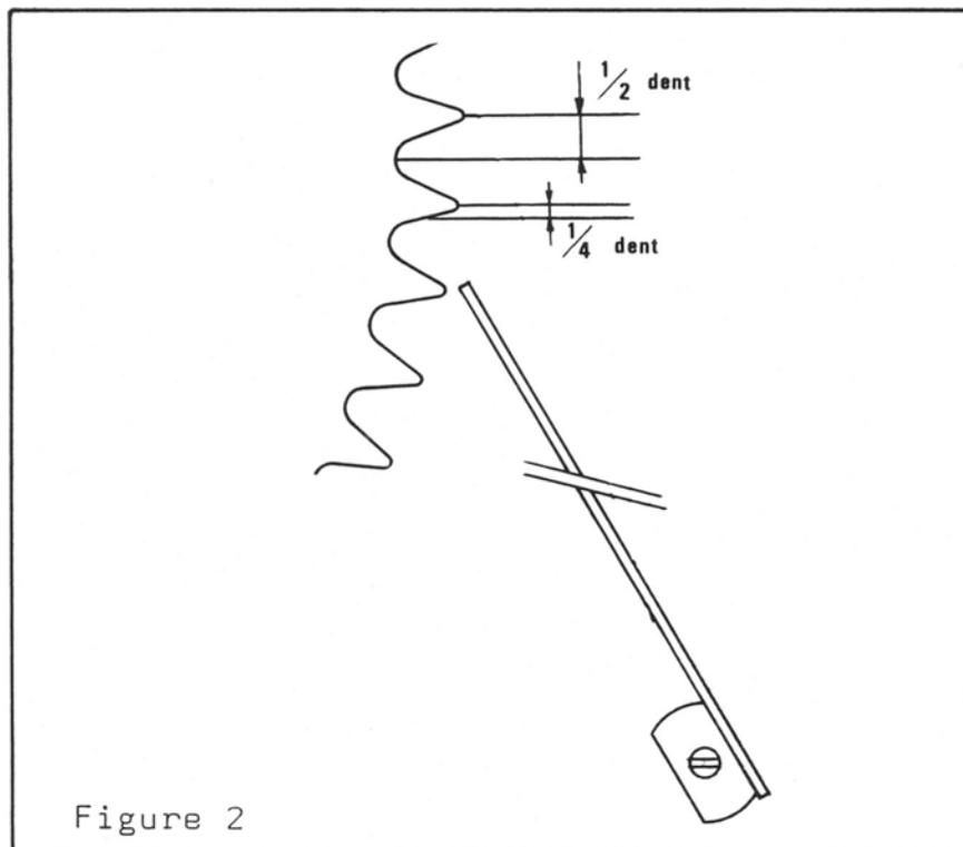
**9.3.** If the backlash has to be modified, turn the eccentric for motor in the direction suitable to the required correction.
