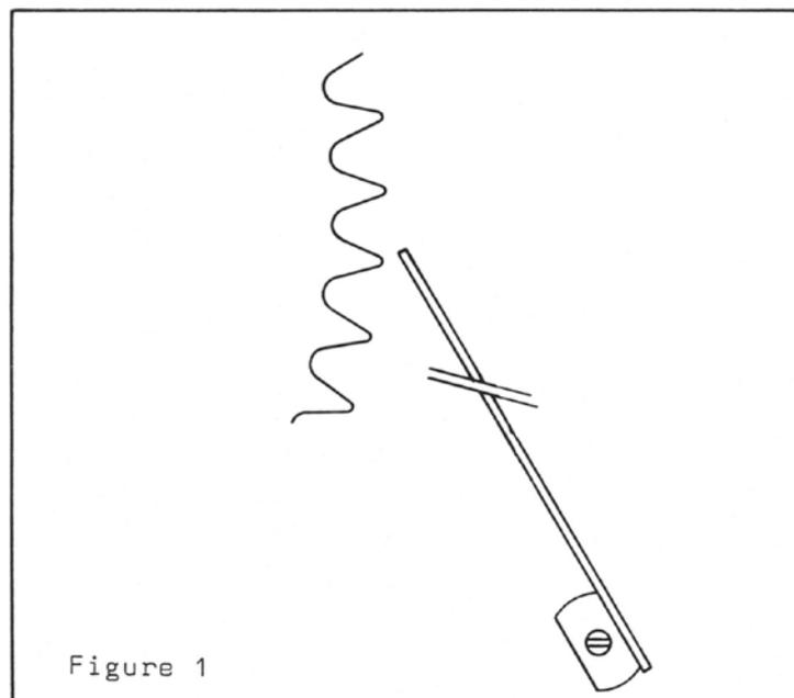
**9.1.** Adjust the retaining click into position shown by figure 1, the end of the click to be used as guiding-mark to observe the movement of the second wheel.
