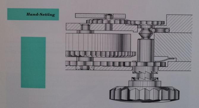
On pulling out the winding crown the winding stem spring gives and bears against the other face of the double cone, thus maintaining the stem in the position which allows engagement of the setting wheel with the motion work, thus setting the hands.
