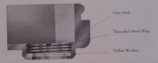
Should it be necessary to repair or alter the case, it is essential that the steel ring and Teflon washer be removed if soldering is to be carried out.
