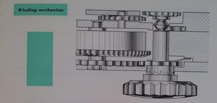
On winding the watch, the clutch wheel which turns with the crown and stem, drives the winding pinion which in turn drives the ratchet wheel fitted on the barrel arbor.
