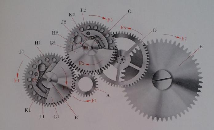
The rotor pinion A revolves in the direction of the arrow F1; it drives the upper winding wheel G2 in the direction of the arrow F2 and the upper winding wheel G1 in the direction of the arrow F3.
