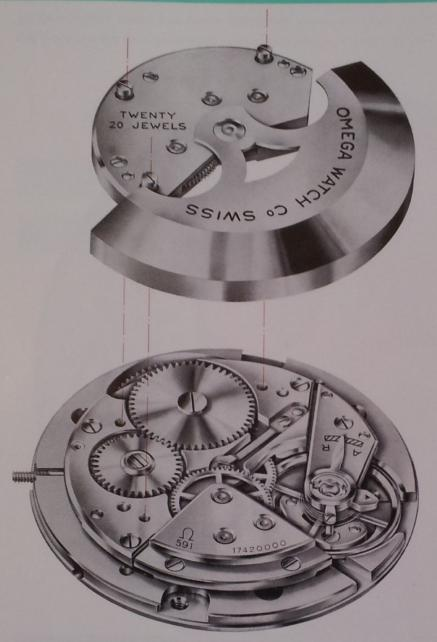
The self winding mechanism forms an independent assembly and is fitted on the barrel bridge by three screws. This arrangement permits simultaneous production of both movement and automatic assembly.
