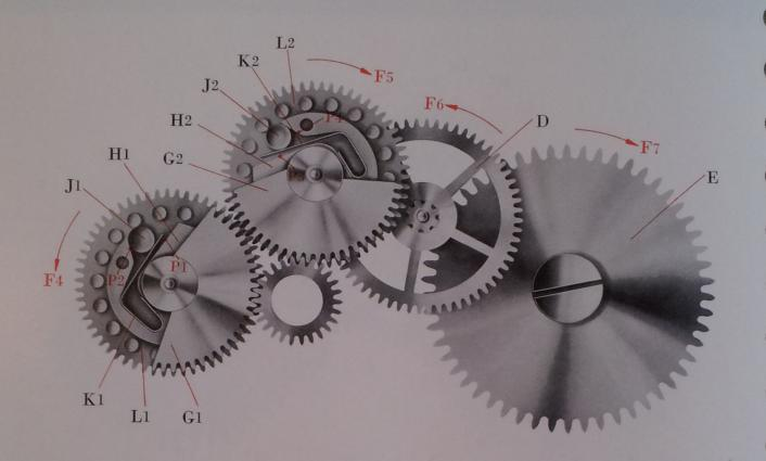
On winding the watch by hand the ratchet wheel E turns in the direction of the arrow F7 and drives through its pinion the ratchet wheel driving gear D in the direction of the arrow F6. This wheel meshing with the pinion of the lower winding wheel L2 causes it to turn in the direction of the arrow F5 which in turn drives the winding wheel L1 in the direction of the arrow F4.
