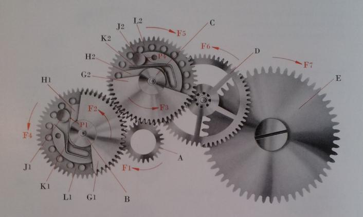
The rotor pinion A turns in the direction of the arrow F1; it drives the upper winding wheel G1 in the direction of the arrow F2 and the upper winding wheel G2 in the direction of the arrow F3.
