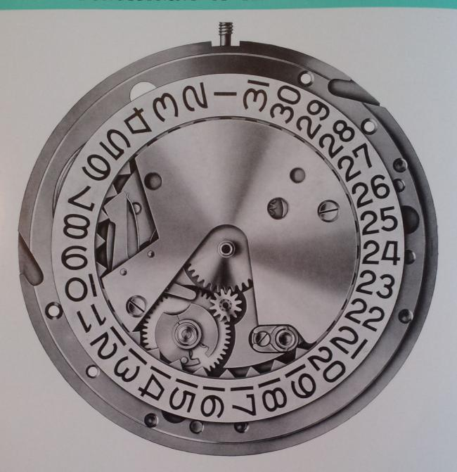
The hour wheel having 36 teeth meshes with the upper half of the double setting wheel having 12 teeth, the lower half having eight teeth meshes with the date indicator driving wheel which performs a complete revolution every 24 hours.
