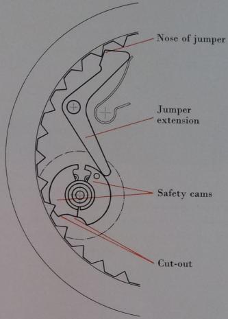
On passing from one tooth to the next the date jumper extension will pass inside the safety cam cut out so as to allow the nose of the jumper to lift over the indicator teeth.
