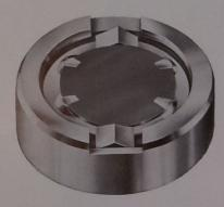
This rotation causes the two extension pieces to line up with the slots in the setting, thus permitting easy removal of endstone and retaining piece.
