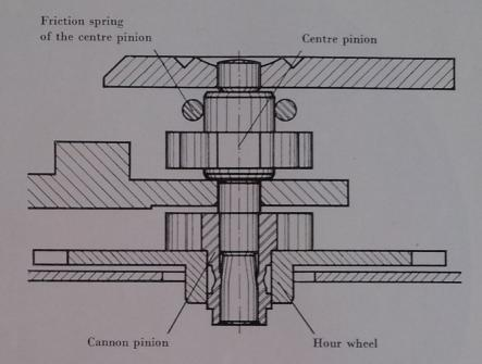
When fitting the friction spring it is important that the ends touch neither the barrel bridge nor the leaves of the centre pinion.
